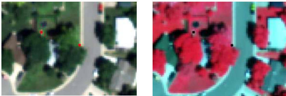
Fig 1) Left: natural color image with two sample points. Right: same image as on the left in infra-red to highlight vegetation.
